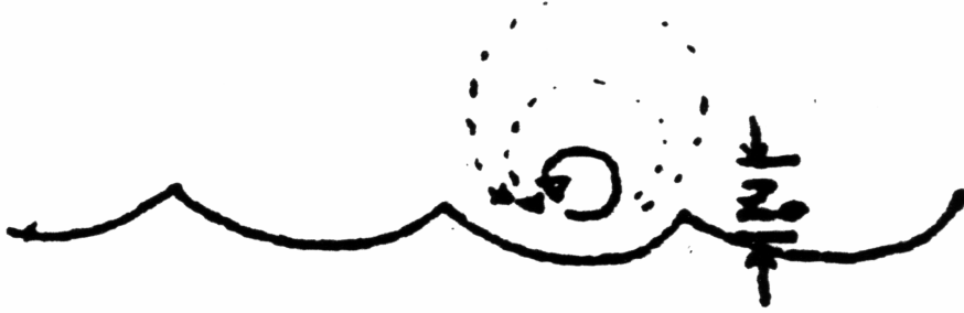
Figure 5.46. Flow eddies associated with surface roughness.
